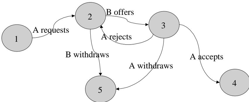
Figure 1: State Diagram of the proposed negotiation protocol
