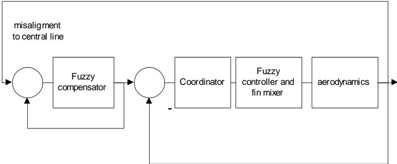
**Figure 1:** Missile pitch guidance loop
