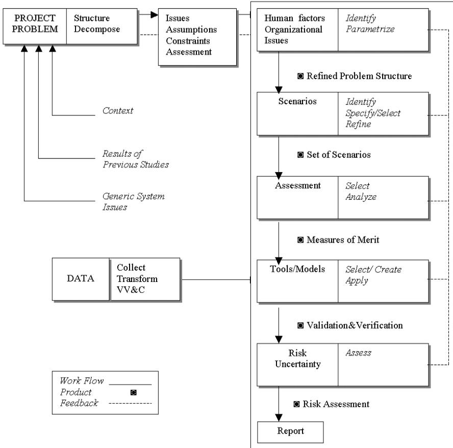
Figure 1: Methodology for management of a project life cycle.
