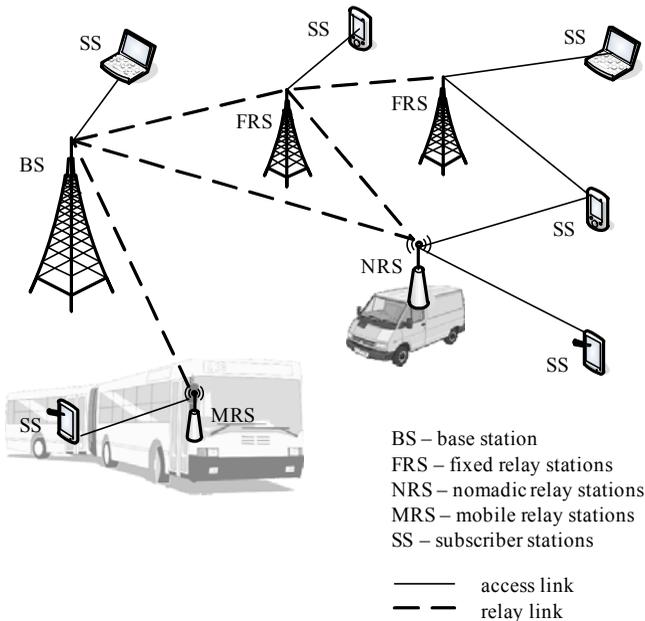
Figure 2: The structure of an IEEE 802.16j WMN.
