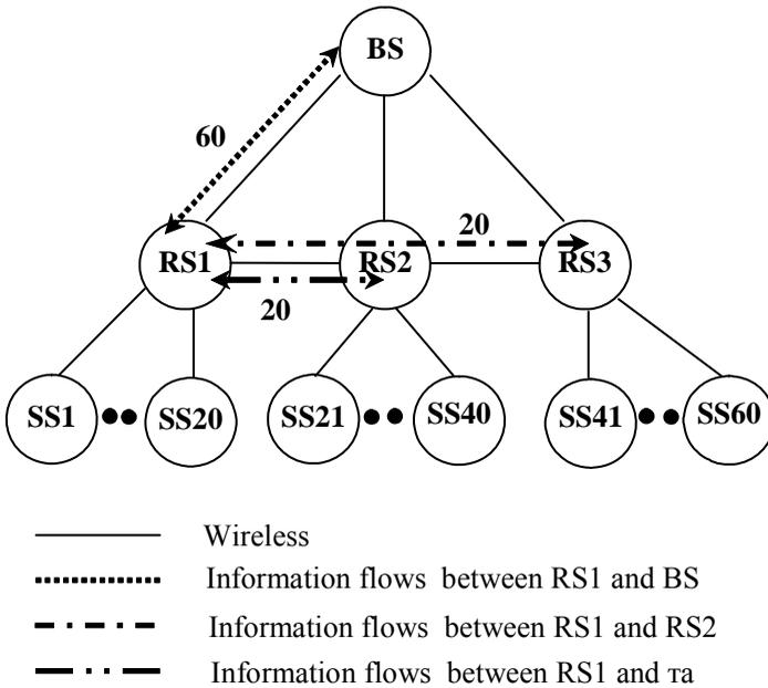
Figure 3: Network structure and directions of information flows.
