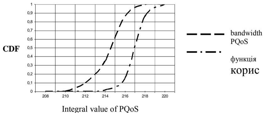
Figure 5: Integral value of PQoS undersign of different methods maximization network utility.
