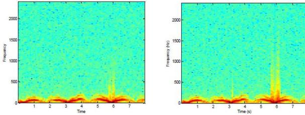
Figure 6: STFT spectrograms of signals from flying drone.
