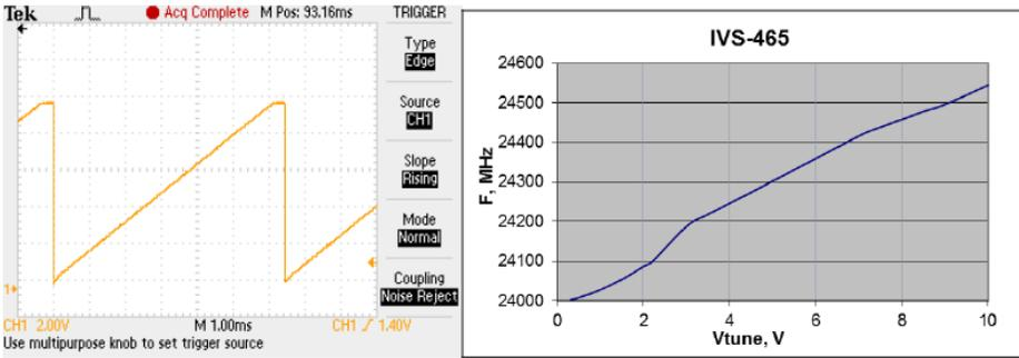
**Figure 3: MyRIO FPGA saw tooth control voltage and radar VCO output frequency**
