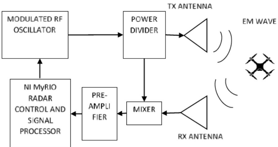
Figure 1: Block diagram of K band radar experimental setup.
