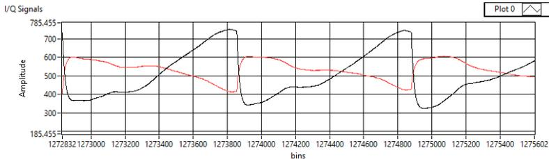
Figure 8: I/Q signals at the output of radar module, LFM transmission (frame 1243), representing data between bins 1272832 and 1273856.
