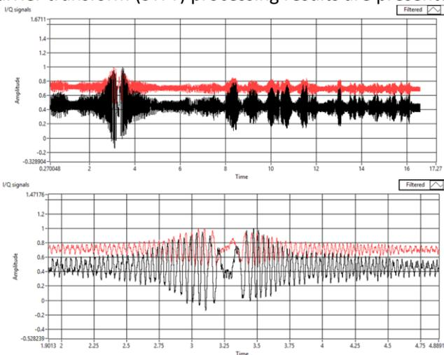
**Figure 4: Drone I/Q signals in radar CW mode of operation.**
