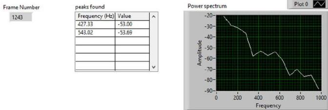
**Figure 9: Results from FFT processing of flying drone beat frequency signal in frame 1243.**
