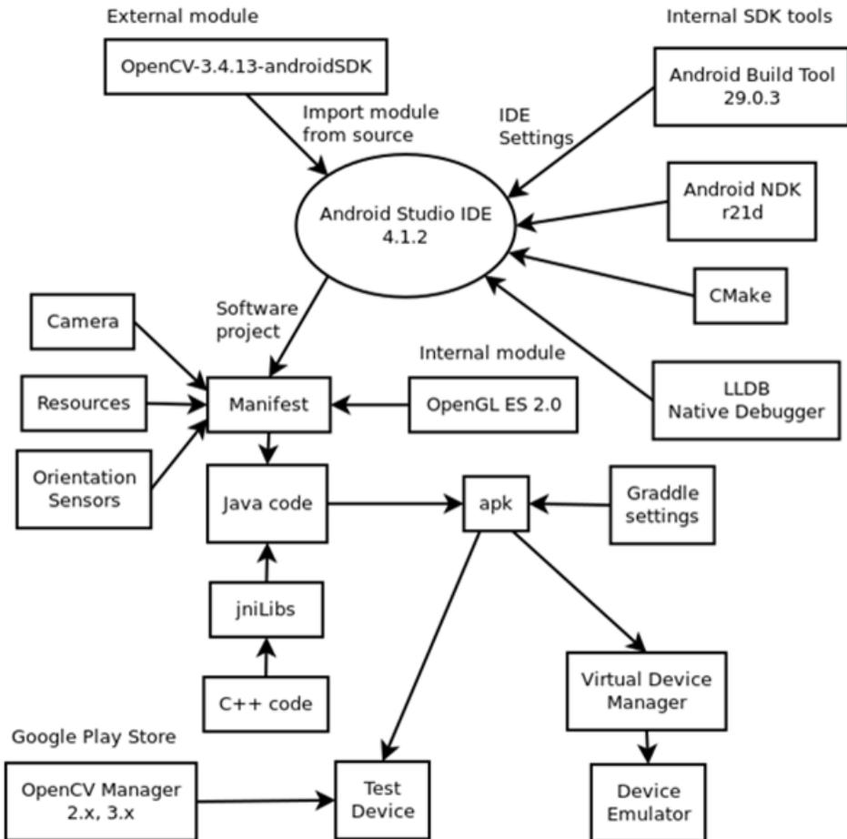
Figure 5: Software architecture of a mobile application with capabilities for reflecting augmented reality.
